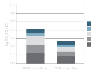
coating 1m<sup>2</sup> of steel with a thickness of 1 mm \*Cradle-to-gate carbon footprint assessment - partial product life cycle from resource extraction to the factory gate exit. **Courtesy of DSM**  Substrate heating Coating production Epoxy resin Resin Pigment
